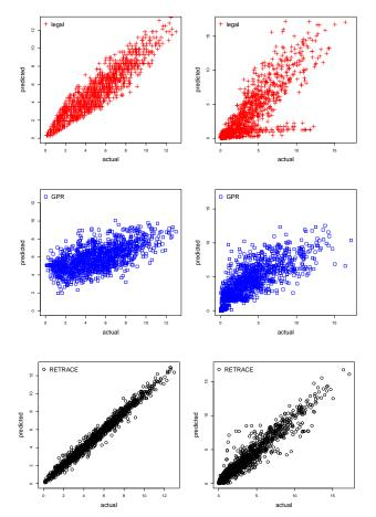
Figure 4: Comparison of travel-times in minute between Legal, GPR, and RETRACE (left column: Grid25, right column: Kyoto). The horizontal axis is the actual travel time, while the vertical axis is the predicted time.
