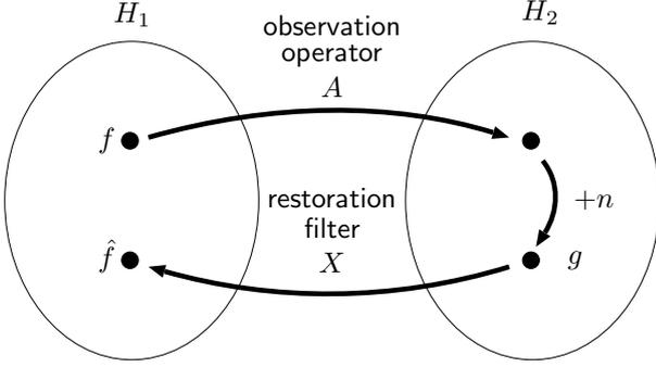
**Fig. 1.** Formulation of image restoration problem.  $f$  is the unknown original image.  $A$  is the observation operator.  $g$  is the observed image.  $n$  is the additive noise.  $X$  is a restoration filter.  $\hat{f}$  is a restored image.
