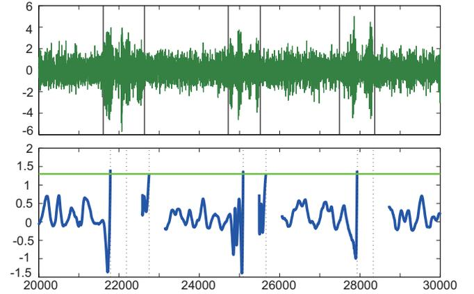
Figure 6: The raw time-series data of the speech dataset (top) and the change-detection score (2.1) of the proposed method (bottom).
